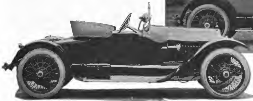
New Stutz roadster with rear deck and tank carried on the rear of the frame. Carrying space is provided beneath the seat and under the deck
